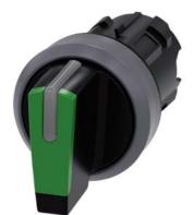
Selector switch, illuminable, 22 mm, round, plastic with metal front ring, green, selector switch, short, 3 switch positions I>O<II, momentary contact type, actuating angle  $2x45^{\circ}$ , 10:30h/12h/13:30h, with laser labeling, upper case
