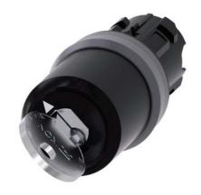
Key-operated switch IKON, 22 mm, round, plastic with metal front ring, lock number 360012K1, with 2 keys, 2 switch positions O-I, latching, actuating angle 90°, 10:30h/13:30h, key removal O+I, with laser labeling, upper case and lower case, always upper case at the beginning of the word
