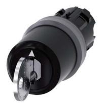
Key-operated switch IKON, 22 mm, round, plastic with metal front ring, lock number 360012K1, with 2 keys, 3 switch positions I-O<II, left latching, right momentary contact type, actuating angle 2x45°, 10:30h/12h/13:30h, key removal O+I, with laser labeling, inscription or symbol Customer-specific selection with SIRIUS ACT configurator (CIN)
