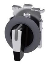
Selector switch, illuminable, 30 mm, round, Metal, matte, white, selector switch, long, front ring for flush installation, 3 switch positions I>O<II, momentary contact type, actuating angle 2x45°, 10:30h/12h/13:30h, with laser labeling, upper case
