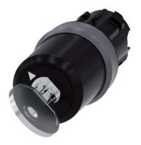
Key-operated switch BKS, 22 mm, round, plastic with metal front ring, Lock No. E7 (VW), without key, 2 switch positions O-I, latching, actuating angle  $90^{\circ}$ , 10:30h/13:30h, key removal O+I, with laser labeling, lower case
