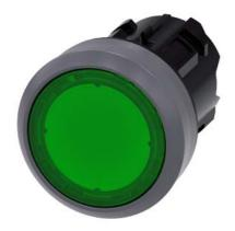
Illuminated pushbutton, 22 mm, round, plastic with metal front ring, green, pushbutton, flat, latching, Push-to-release mechanism, with laser labeling, symbol number according to, ISO 7000 or IEC 60417
