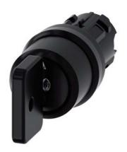
Key-operated switch O.M.R, 22 mm, round, plastic, lock number 73034, black, with 2 keys, 3 switch positions I-O-II, latching, actuating angle 2x45°, 10:30h/12h/13:30h, key removal O, with laser labeling, lower case
