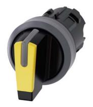
Selector switch, illuminable, 22 mm, round, plastic with metal front ring, yellow, selector switch, short, 3 switch positions I-O<II, left latching, right momentary contact type, actuating angle 2x45°, 10:30h/12h/13:30h, with laser labeling, upper case
