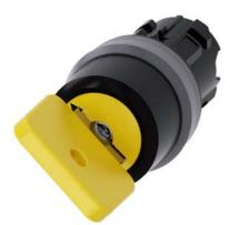
Key-operated switch O.M.R, 22 mm, round, plastic with metal front ring, lock number 73033, yellow, with 2 keys, 2 switch positions O-I, latching, actuating angle 90°, 10:30h/13:30h, key removal O, with laser labeling, upper case and lower case, always upper case at the beginning of the word
