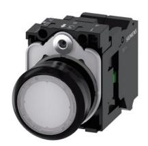
Illuminated pushbutton, 22 mm, round, plastic, white, pushbutton, flat, momentary contact type, with holder, 1NO, LED module with integrated LED 230 V AC, spring-type terminal, with laser labeling, lower case
