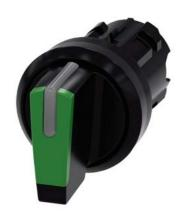
Selector switch, illuminable, 22 mm, round, plastic, green, selector switch, short, 3 switch positions I-O-II, latching, actuating angle 2x45°, 10:30h/12h/13:30h, with laser labeling, upper case and lower case, always upper case at beginning of line
