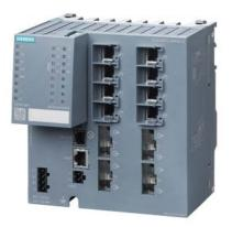
SCALANCE XM408-4C; managed modular IE switch; 8x 10/100/1000 Mbit/s RJ45; 4x 100/1000 Mbps ST-/SC- pluggable as combo ports; in total 8 ports can be used; expandable to 24 ports electrical or optical; assembly: DIN rail/S7 mounting rail, PROFINET IO device; redundancy functions; office features (RSTP, VLAN, IGMP,...); C-PLUG in scope of supply; layer 3 integrated.
