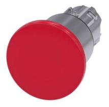
Mushroom pushbutton, 22 mm, round, metal, shiny, red, 40 mm, 3 switch positions, latches after pushing in, unlatches by pull-to-unlatch mechanism to center position, after pulling out the button Retraction to center position, with laser labeling, inscription or symbol Customer-specific selection with SIRIUS ACT configurator (CIN)
