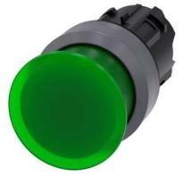
Illuminated mushroom pushbutton, 22 mm, round, plastic with metal front ring, green, 30 mm, momentary contact type, with laser labeling, inscription or symbol Customer-specific selection with SIRIUS ACT configurator (CIN)
