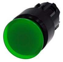
Illuminated mushroom pushbutton, 22 mm, round, plastic, green, 30 mm, latching, pull-to-unlatch mechanism, with laser labeling, upper case and lower case, always upper case at beginning of line
