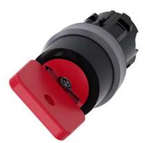
Key-operated switch O.M.R, 22 mm, round, plastic with metal front ring, lock number 73037, red, with 2 keys, 2 switch positions O-I, latching, actuating angle 90°, 10:30h/13:30h, key removal O+I, with laser labeling, upper case and lower case, always upper case at beginning of line
