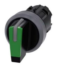
Selector switch, illuminable, 22 mm, round, plastic with metal front ring, green, selector switch, short, 3 switch positions I-O-II, latching, actuating angle  $2x45^{\circ}$ , 10:30h/12h/13:30h, with laser labeling, upper case and lower case, always upper case at the beginning of the word
