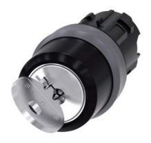
RONIS key-operated switch, 22 mm, round, plastic with metal front ring, lock number SB30, with 2 keys, 2 switch positions O-I, latching, actuating angle 90°, 10:30h/13:30h, key removal I, possible special locks: SB31, 421, 455, with laser labeling, upper case and lower case, always upper case at beginning of line
