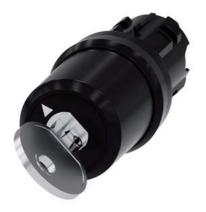
key-operated switch Siemens, 22 mm, round, plastic, lock no. LSG1, with 2 keys, 2 switch positions O<I, momentary contact type, actuating angle 45°, 10:30h/12h, key removal O, with laser labeling, lower case
