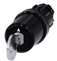
key-operated switch Siemens, 22 mm, round, plastic, lock number SSG10, with 2 keys, 3 switch positions I-O<II, left latching, momentary contact type on the right, actuating angle  $2x45^{\circ}$ , 10:30h/12h/13:30h, key removal I, with laser labeling, lower case
