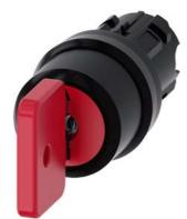
Key-operated switch O.M.R, 22 mm, round, plastic, lock number 73037, red, with 2 keys, 3 switch positions I>O<II, momentary contact type, actuating angle 2x45°, 10:30h/12h/13:30h, key removal O, with laser labeling, lower case
