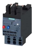
Overload relay 27...32 A Thermal For motor protection Size S0, Class 10 Contactor mounting Main circuit: Spring-type terminal Auxiliary circuit: spring-type terminal Manual-Automatic-Reset
