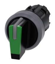
Selector switch, illuminable, 22 mm, round, plastic with metal front ring, green, selector switch, short, 3 switch positions I>O<II, momentary contact on the left, latching on the right, actuating angle 2x45°, 10:30h/12h/13:30h, with laser labeling, upper case
