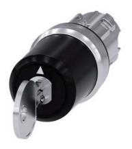
key-operated switch Siemens, 22 mm, round, metal, shiny, lock number SSG10, with 2 keys, 3 switch positions I>O<II, momentary contact on the left, latching on the right, actuating angle 2x45°, 10:30h/12h/13:30h, key removal O, with laser labeling, inscription or symbol customer-specific selection with SIRIUS ACT configurator (CIN)
