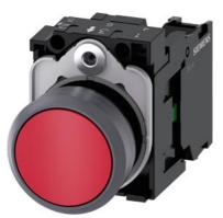
Pushbutton, 22 mm, round, plastic with metal front ring, red, pushbutton, flat, momentary contact type, with holder, 1 NO, screw terminal, with laser labeling, inscription or symbol Customer-specific selection with SIRIUS ACT configurator (CIN)
