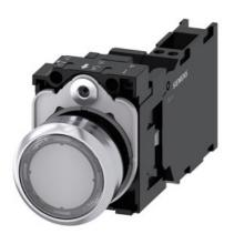
Illuminated pushbutton, 22 mm, round, Metal, shiny, transparent, pushbutton, flat, momentary contact type, with holder, 1 NO+1 NC, LED module with integrated LED 230 V AC, spring-type terminal, with laser labeling, upper case
