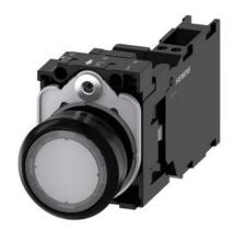
Illuminated pushbutton, 22 mm, round, plastic, clear, pushbutton, flat, momentary contact type, with holder, 1 NO+1 NC, LED module with integrated LED 110 V AC, spring-type terminal, with laser labeling, symbol number according to, ISO 7000 or IEC 60417
