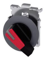
Selector switch, illuminable, 30 mm, round, Metal, matte, red, selector switch, long, front ring for flush installation, 2 switch positions O<I, momentary contact type, Actuating angle 45°, 10:30h/12h, Z=50-unit packaging
