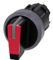
Selector switch, illuminable, 22 mm, round, plastic with metal front ring, red, selector switch, short, 3 switch positions I>O<II, momentary contact type, actuating angle  $2x45^{\circ}$ , 10:30h/12h/13:30h, Z=50-unit packaging
