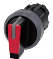
Selector switch, illuminable, 22 mm, round, plastic with metal front ring, red, selector switch, short, 3 switch positions I-O<II, left latching, right momentary contact type, actuating angle 2x45°, 10:30h/12h/13:30h, with laser labeling, upper case and lower case, always upper case at beginning of line
