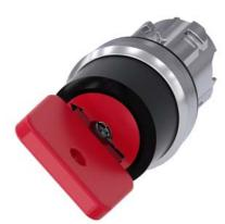
Key-operated switch O.M.R, 22 mm, round, metal, shiny, lock number 73037, red, with 2 keys, 2 switch positions O-I, latching, actuating angle 90°, 10:30h/13:30h, key removal O, with laser labeling, lower case
