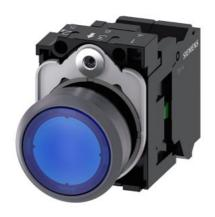
Illuminated pushbutton, 22 mm, round, plastic with metal front ring, blue, pushbutton, flat, momentary contact type, with holder, 1NO, LED module with integrated LED 24 V AC/DC, spring-type terminal, with laser labeling, upper case and lower case, Always upper case at the beginning of the word
