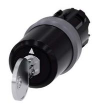
Key-operated switch BKS, 22 mm, round, plastic with metal front ring, lock number S1, with 2 keys, 3 switch positions I-O-II, latching, actuating angle  $2x45^{\circ}$ , 10:30h/12h/13:30h, key removal O, with laser labeling, inscription or symbol Customer-specific selection with SIRIUS ACT configurator (CIN)
