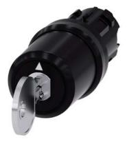
key-operated switch Siemens, 22 mm, round, plastic, special lock, with 2 keys, 3 switch positions I-O-II, latching, actuating angle  $2x45^\circ,\,10:30h/12h/13:30h,$  key removal O
