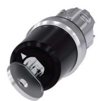
key-operated switch Siemens, 22 mm, round, metal, shiny, lock no. STGH10, with 2 keys, 2 switch positions O<I, momentary contact type, actuating angle 45°, 10:30h/12h, key removal O, with laser labeling, upper case and lower case, always upper case at beginning of line
