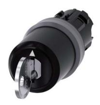
Key-operated switch IKON, 22 mm, round, plastic with metal front ring, lock number 360012K1, with 2 keys, 3 switch positions I-O-II, latching, actuating angle 2x45°, 10:30h/12h/13:30h, Key removal I+O+II, with laser labeling, inscription or symbol Customer-specific selection with SIRIUS ACT configurator (CIN)
