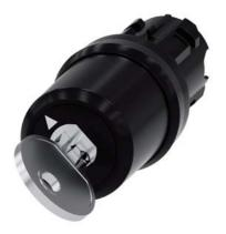
key-operated switch Siemens, 22 mm, round, plastic, lock no. LSG1, with 2 keys, 2 switch positions O<I, momentary contact type, actuating angle  $45^\circ,\,10:30h/12h,$  key removal O, with laser labeling, upper case
