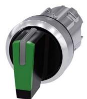
Selector switch, illuminable, 22 mm, round, metal, shiny, green, selector switch, short, 3 switch positions I-O-II, latching, actuating angle 2x45°, 10:30h/12h/13:30h, Z=50-unit packaging
