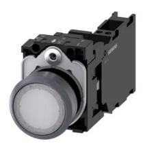
Illuminated pushbutton, 22 mm, round, plastic with metal front ring, white, pushbutton, flat, momentary contact type, with holder, 1 NO+1 NC, LED module with integrated LED 24 V AC/DC, spring-type terminal, with laser labeling, symbol number according to, ISO 7000 or IEC 60417
