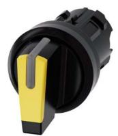
Selector switch, illuminable, 22 mm, round, plastic, yellow, selector switch, short, 3 switch positions I-O-II, latching, actuating angle  $2x45^{\circ}$ , 10:30h/12h/13:30h Z=50-unit packaging
