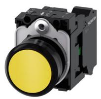
Pushbutton, 22 mm, round, plastic, yellow, pushbutton, flat, momentary contact type, with holder 1 NO, spring-type terminal, with laser labeling, symbol number according to, ISO 7000 or IEC 60417
