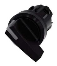
Illuminable selector switch, 22 mm, round, plastic, black, Selector switch long, 2 switch positions O-I, latching, actuating angle 90°, 10:30 /13:30, Z=50-unit packaging
