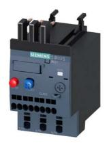
Overload relay 0.35...0.50 A Thermal For motor protection Size S00, Class 10 Contactor mounting Main circuit: Spring-type terminal Auxiliary circuit: spring-type terminal Manual-Automatic-Reset
