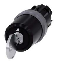
key-operated switch Siemens, 22 mm, round, plastic with metal front ring, lock number SSG10, with 2 keys, 3 switch positions I-O-II, latching, actuating angle 2x45°, 10:30h/12h/13:30h, key removal I, with laser labeling, upper case and lower case, always upper case at beginning of line
