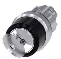
RONIS key-operated switch, 22 mm, round, metal, shiny, lock number SB30, with 2 keys, 2 switch positions O<I, momentary contact type, Actuating angle 45°, 10:30h/12h, key removal O, possible special locks: SB31, 421, 455, with laser labeling, upper case and lower case, always upper case at the beginning of the word
