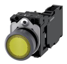
Illuminated pushbutton, 22 mm, round, plastic with metal front ring, yellow, pushbutton, flat, momentary contact type, with holder, 1 NO+1 NC, LED module with integrated LED 110 V AC, screw terminal
