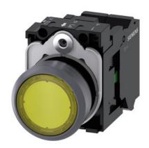
Illuminated pushbutton, 22 mm, round, plastic with metal front ring, yellow, pushbutton, flat, momentary contact type, with holder, 1NO, LED module with integrated LED 24 V AC/DC, spring-type terminal, with laser labeling, symbol number according to, ISO 7000 or IEC 60417
