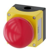
Enclosure for command devices 22 mm, round, Enclosure material metal, Enclosure top part yellow, 1 control point metal, Control point in center, A=EMERGENCY STOP palm pushbutton, red, positive latching, pull-to-unlatch mechanism, 1 NC, 1 NO, screw terminal, Floor mounting
