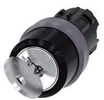
RONIS key-operated switch, 22 mm, round, plastic with metal front ring, special lock, with 2 keys, 2 switch positions O<I, momentary contact type, Actuating angle 45°, 10:30h/12h, key removal O, possible special locks: SB31, 421, 455
