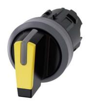
Selector switch, illuminable, 22 mm, round, plastic with metal front ring, yellow, selector switch, short, 3 switch positions I>O<II, momentary contact on the left, latching on the right, actuating angle 2x45°, 10:30h/12h/13:30h, with laser labeling, inscription or symbol Customer-specific selection with SIRIUS ACT configurator (CIN)
